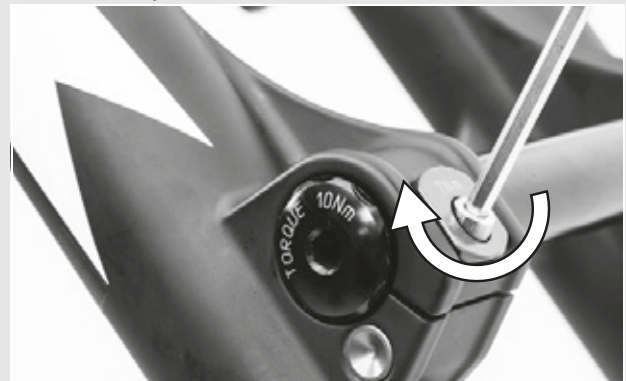
Figure 28: Tightening the axle
