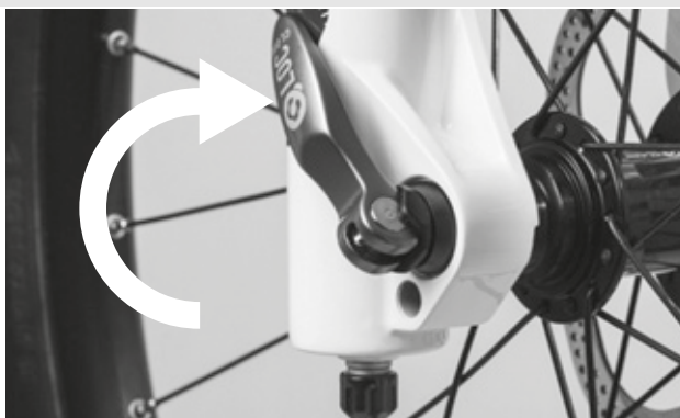
Figure 38: Closing the quick release
