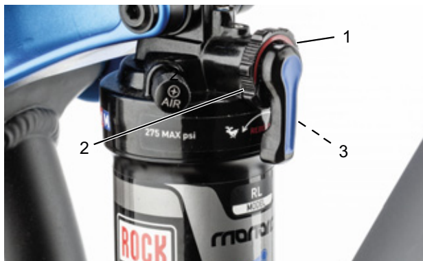
Figure 77: Setting the rebound damper strength on the rear frame damper setting wheel (1)
