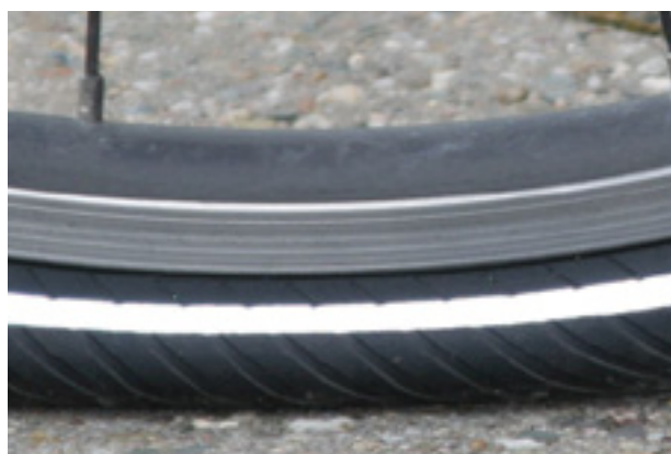
Illustration 104 : Pression largement insuffisante
