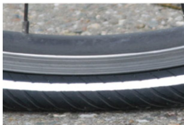
Illustration 79 : Pression largement insuffisante
