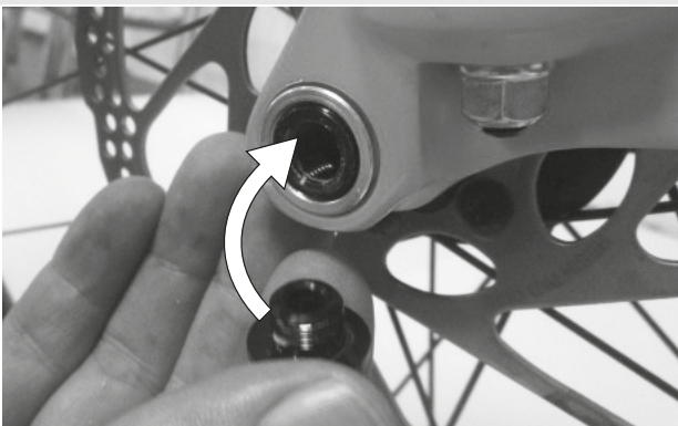
Figure 28: Pushing the quick release lever into the axle
