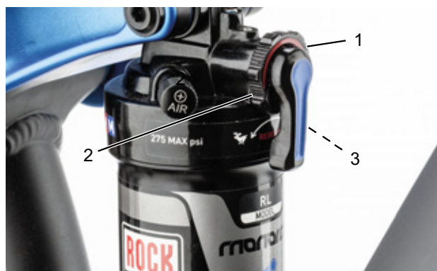
Figure 81: Setting the rebound damper strength on the rear frame damper setting wheel (1)
