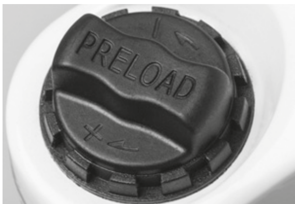
Figure 59: Negative deflection setting wheel on the suspension fork crown
