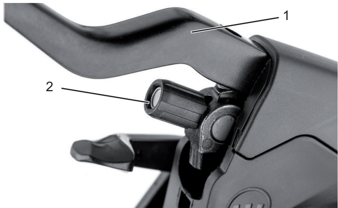
Figure 64: Brake lever (1) of the hydraulically operated rim brake with setting bolt (2)
